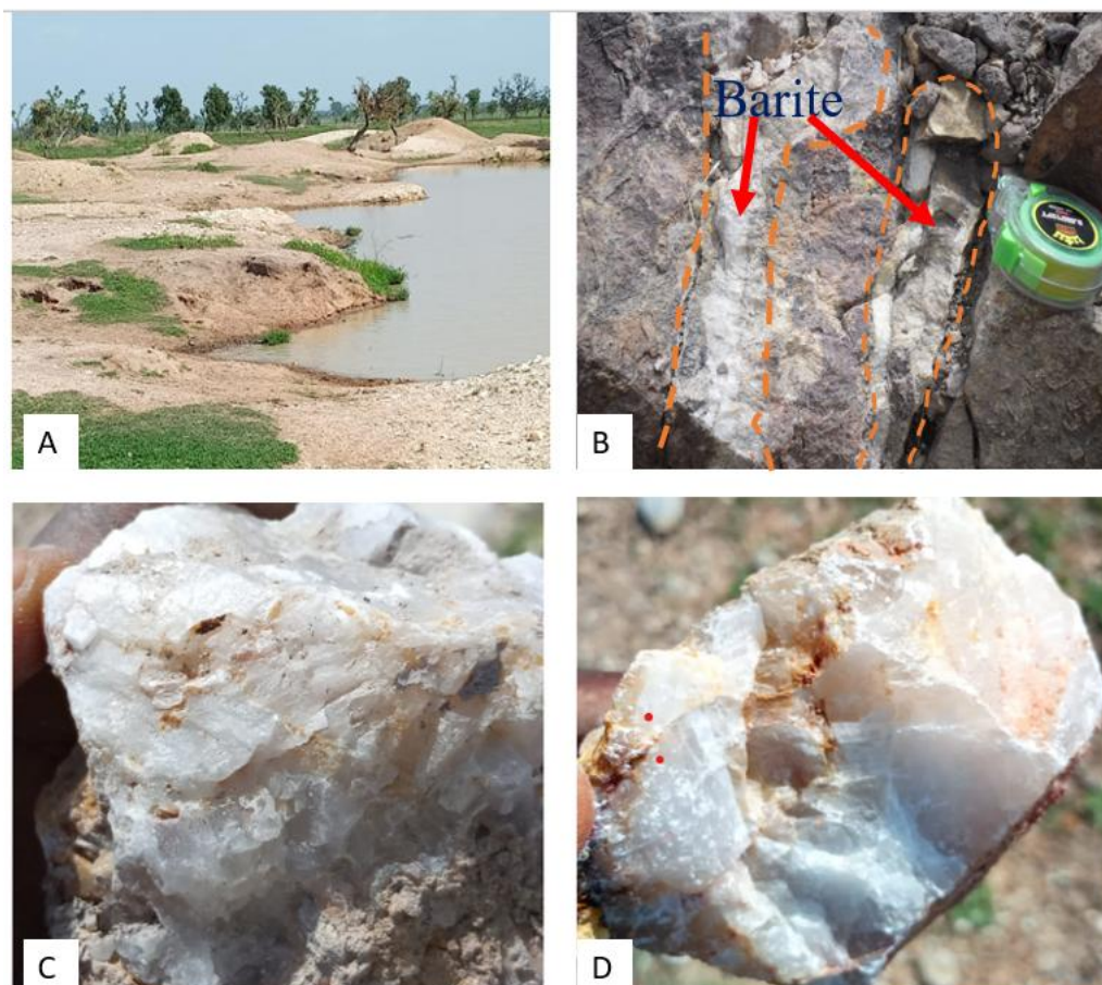
Figure 6: Field Photograph of Didango Barite field (A) Barite mining Pit Filled with Water, (B) Barite Veins in Altered Sandstones, (C and D) Massive Barite with Tints of Ferrous Material
