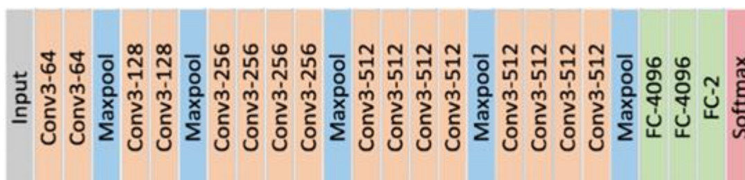
Figure 5: VGG19 Network Structure (Wang et al., 2020)
